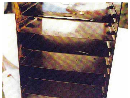
Fig. 2 and 3: Test bearing and pre-heating unit after the FAG FE8 test run: there is no formation of residues on the bearing and the test rig as well as the pre-heating unit
